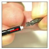
Now flip the applicator around and press the new wax trap in to replace the old one.
